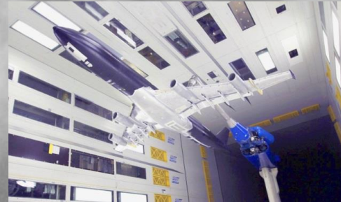
2014 – 2015 Wind tunnel tests Laminar wing & Krueger flap demonstrator
